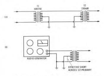
Direct connection across a truly balanced input can result in severe mismatching and test conditions not simulating normal operation of the input circuit.
