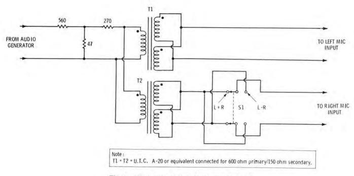
Figure 4E. A coupling unit for stereo tests.
