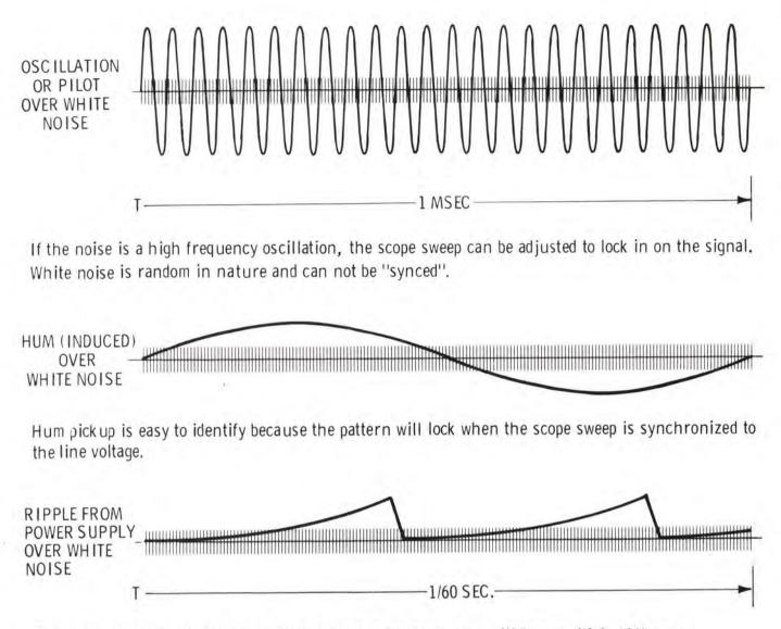
This type of noise will also sync. to the line but it's frequency will be a multiple of the power line frequency.
