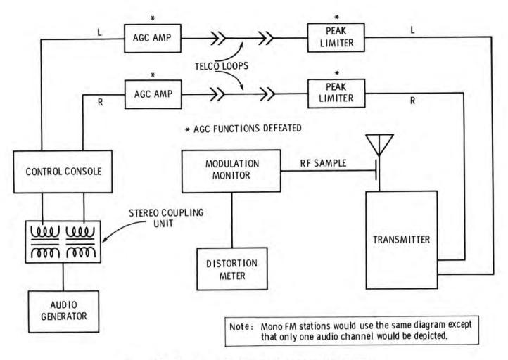
Figure 3A. Sample test equipment connection diagram.
