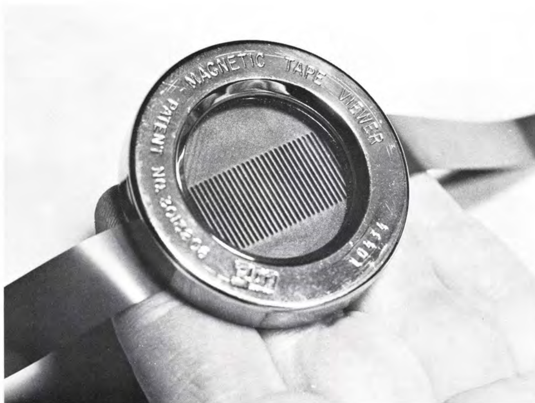
Magnetic pattern as seen with 3M viewer.
