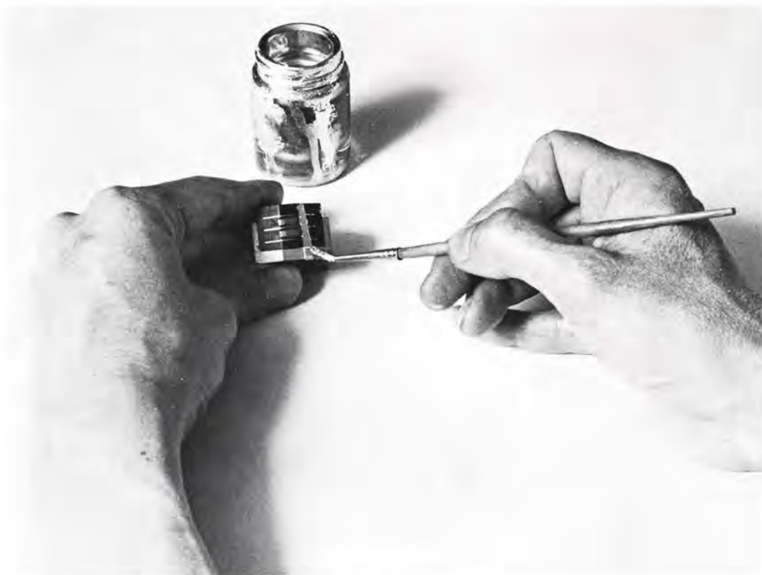
"Painting" a ground with conductive silver paint.
