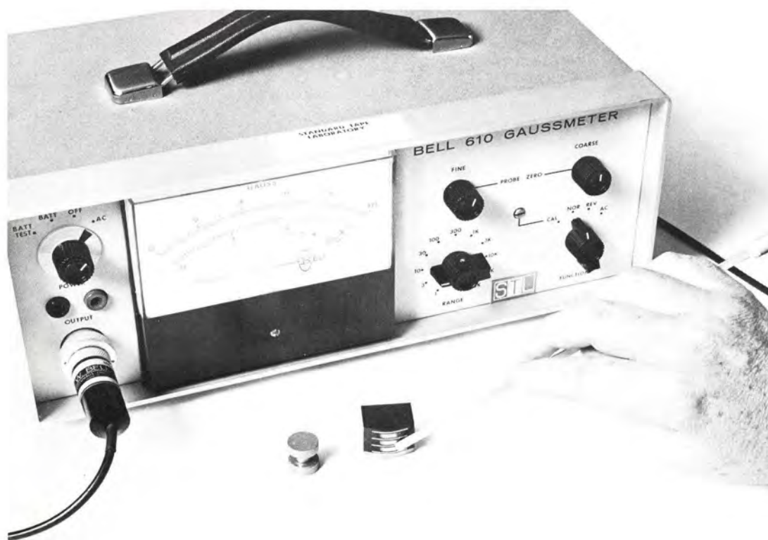
Hall effect Gaussmeter — Note: Head shows almost 5 Gauss field.
