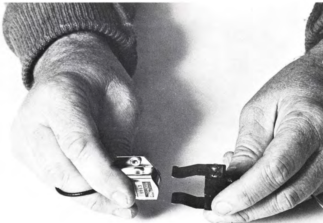
Induction loop jig is held in place by means of spring clips.
