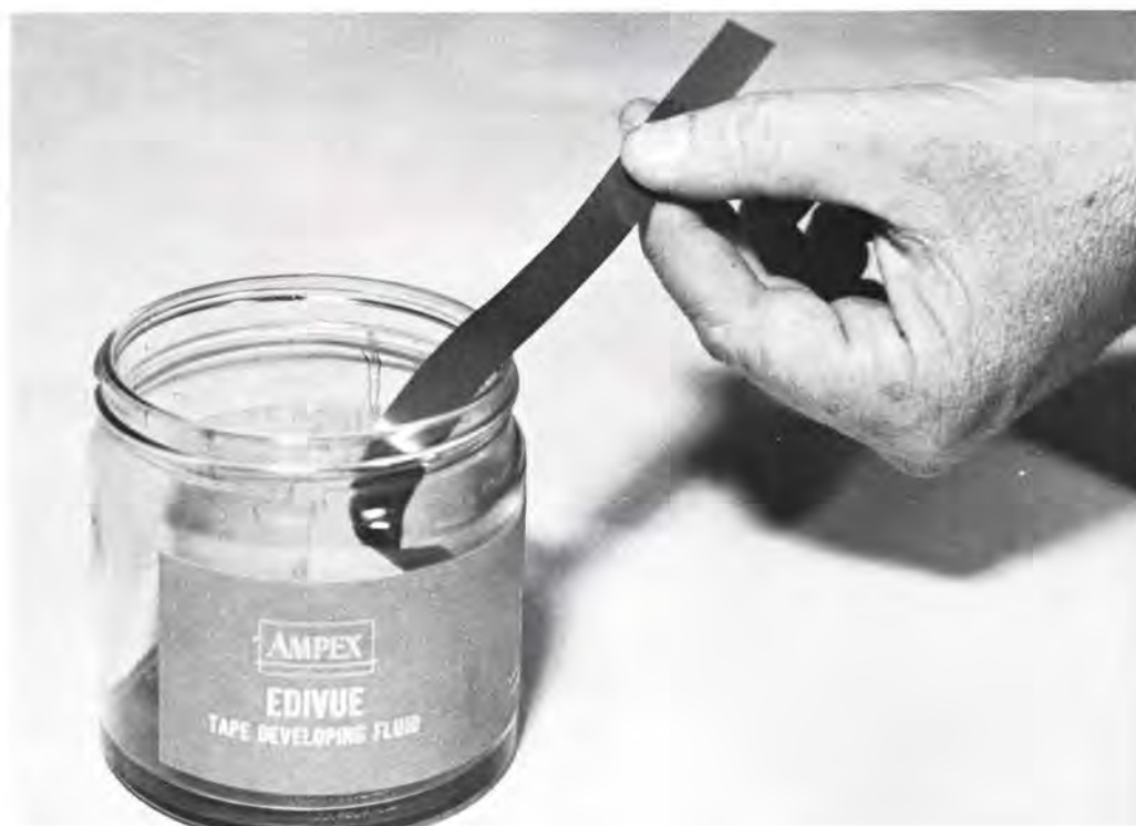
Tape is dipped into indicator fluid.
