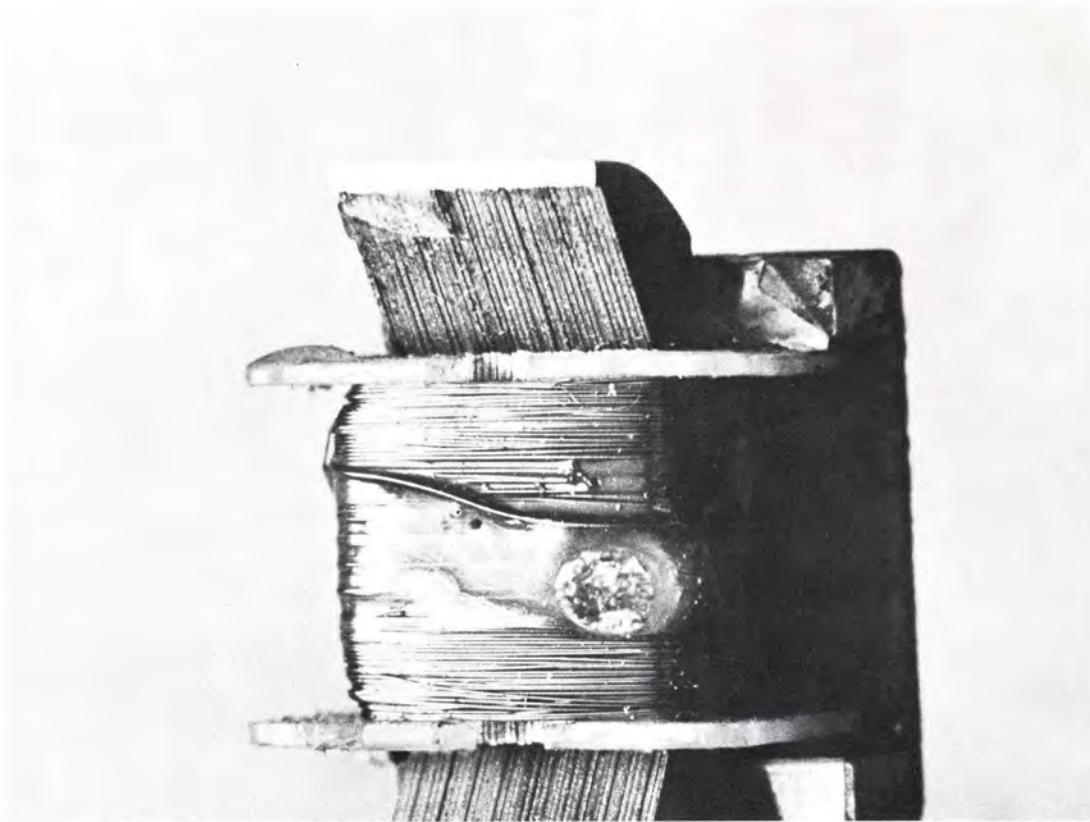
Figure B – Even core depth – head disassembled.
