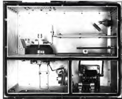
601A DRIVER (IPA) SIMPLIFIED STRIPLINE TUNING
