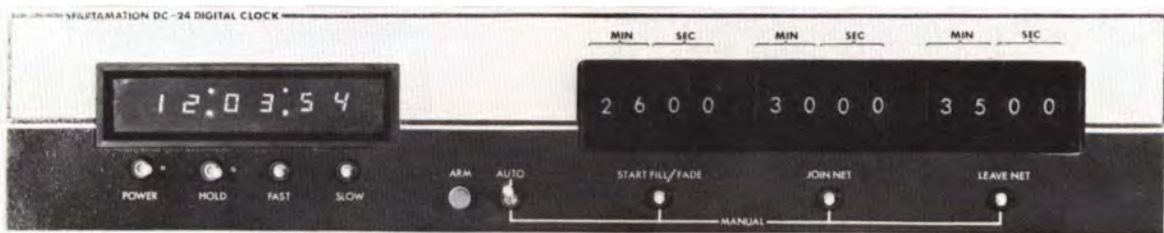
Digital Clock with thumbwheel switches for control of automatic network joining.
