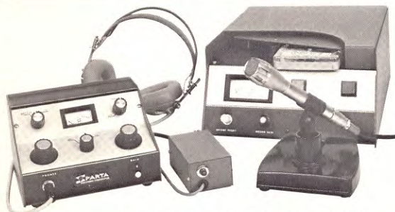
TYPICAL REMOTE BROADCAST ARRANGEMENT Operators' microphone through Channel 1; SPARTA-MATIC® Tape Cartridge playback unit through Channel 2A and roving microphone through Channel 2B.
