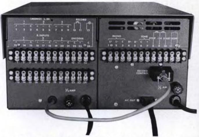
Rear of mono Century Series R/P, showing Record Control inter-connection, AC out of playback to record module, clearly indicated connections.
