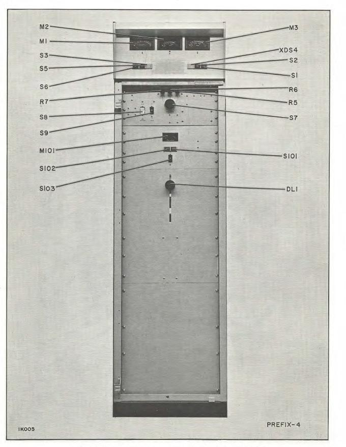
Figure 8. Combining Equipment Cabinet, Electrical Parts, Front View
