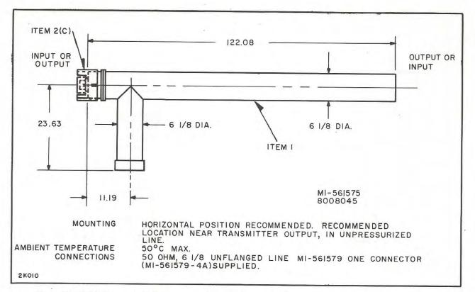
Figure 21. 40 kW Harmonic Filter, Unpressurized, with Item 2 (C) Coupling Attached, Outline Drawing
