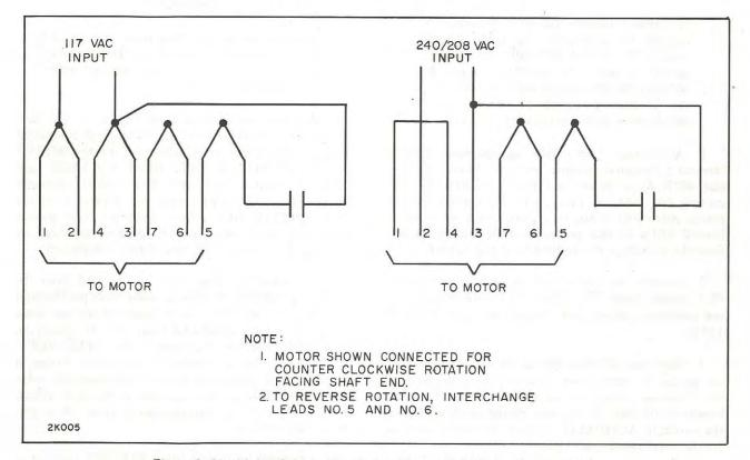
Figure 6. Combining Cabinet Ventilation Motor, 4B1, Wiring Connections
