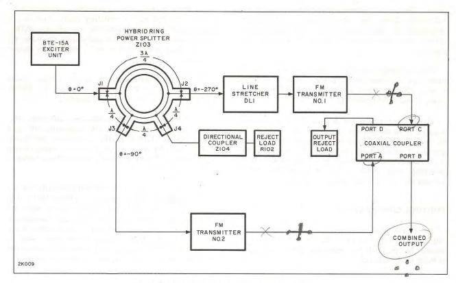
Figure 5. BTF-40E1 Transmitter, Functional Diagram
