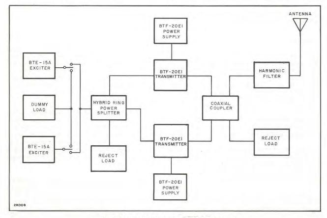
Figure 2. BTF-40E1 Simplified Block Diagram
