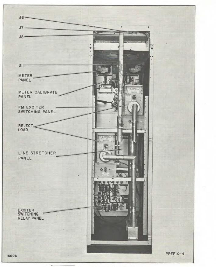
Figure 10. Combining Equipment Cabinet, Rear View
