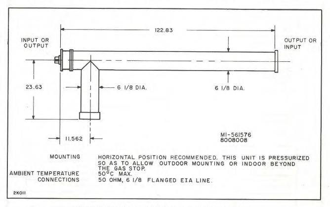
Figure 22. 40 kW Harmonic Filter, Pressurized, Outline Drawing
