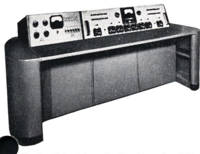
FIG. 6. Television Audio Console. This console is the control center for the audio part of the television program.
