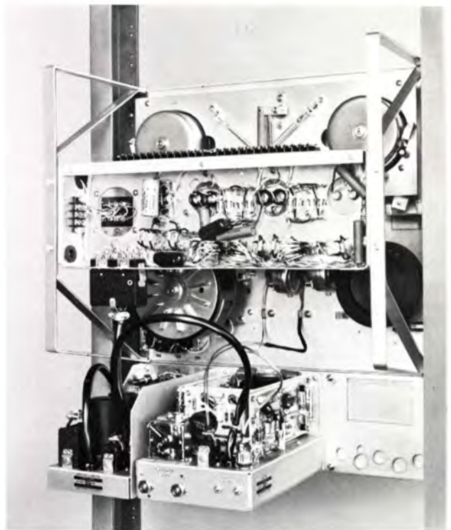
Front and rear views of RT-21B Tape Recorder showing tape transport at top, and control panel below. In rear view the modular control unit is shown at left and amplifier module in center. Space at right supports a second amplifier module for stereo tape operation.
