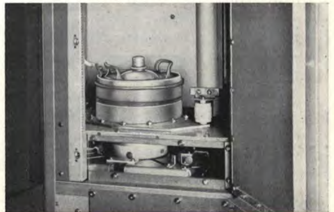
BTF-5D Power Amplifier shown behind hinged front door.
