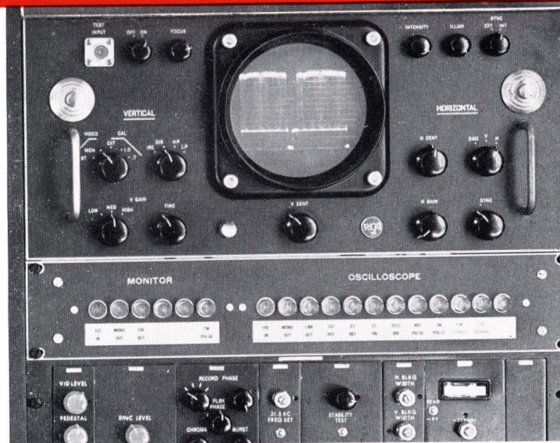
Oscilloscope provides operator with quick check of machine performance. Has built in switching facilities.
