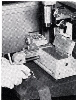
(B) To locate nearest "edit" or "frame" pulse, operator dispenses liquid solution of iron oxide particles to develop magnetic pattern.
