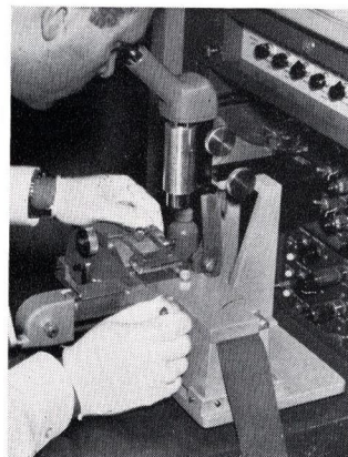
(C) Operator aligns edge of video track on the built-in reticule in order to cut tape halfway between adjacent video tracks.
