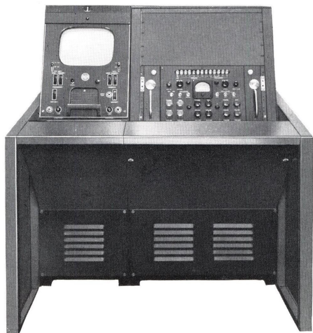
Console Housings, MI-26786 and MI-26787 provide a convenient control center for the TK-26B Color Film Camera Equipment. The 13-inch console to left houses the TM-6C Master Monitor, and 22-inch console housing on right provides mounting of the Processing Amplifier. The camera control panel is mounted in the indented section of the 22-inch console desk.
