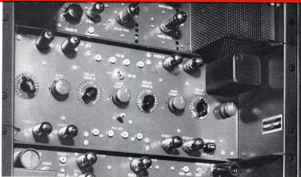
This single chassis is used for manual control of both record and playback quadrature correction in the TR-11. A switch, mounted on the back of the chassis, allows the operator to select playback or record mode.
