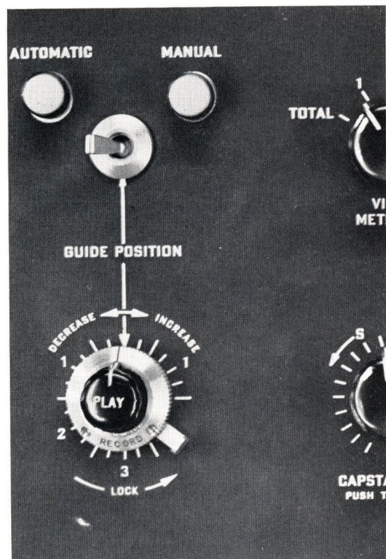
Separate play-record, guide-position controls minimize operator errors.
