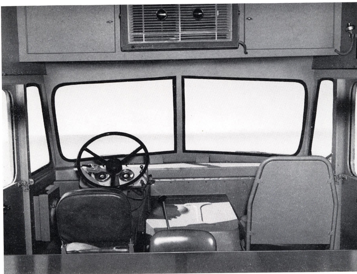
Interior view of mobile unit showing driver's position with built-in air conditioning facilities.
