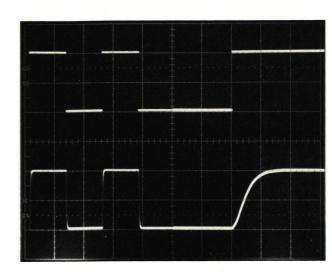
Upper Trace 2KHz Square Wave Input Lower Trace Amplifier Output Left Trace 0.2 ms/div
