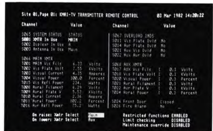
CRT Master Page, derived from Telemetry and Status Pages. Titles, telemetry, and status information may be intermixed from one site as desired.
