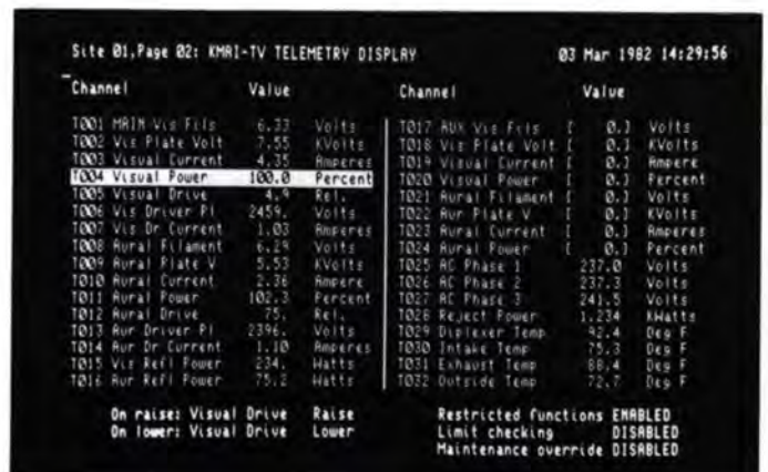
Typical MRC-2 CRT Option Telemetry Page showing 32 channels of telemetry. Channel T004 is in "Take Command" mode, with control functions for channel indicated in lower left hand corner.
