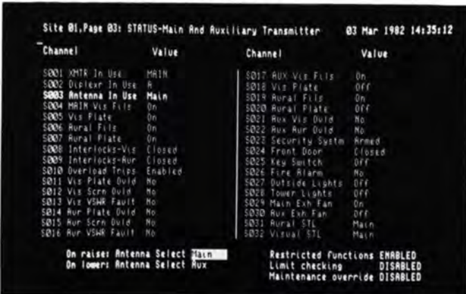
Typical MRC-2 CRT Option Status Page. Note user-generated text, including heading, as well as system status indications.
