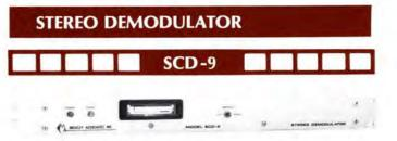
The Model SCD-9 Stereo Demodulator transforms a composite stereo waveform into discrete left and right channels for AM stereo and FM broadcast. Complementary to the SCG-9A Stereo Generator, it includes de-emphasis circuitry, 15 kHz low pass filters, and front panel and stereo indication, with an SPDT relay for external control.
