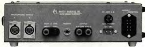
Rear apron of RPA-1. Standard connectors are used for all connections. Note vinyl cushion feet to provide protection in operating and carrying positions.
