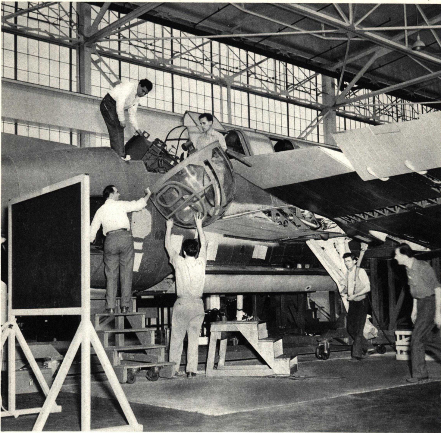
Up goes the plexiglass gun turret to be set behind the pilot's cockpit as the Avenger approaches the end of its final assembly trip. Forward, the canopy fashioned in Tarrytown is already up in place.
