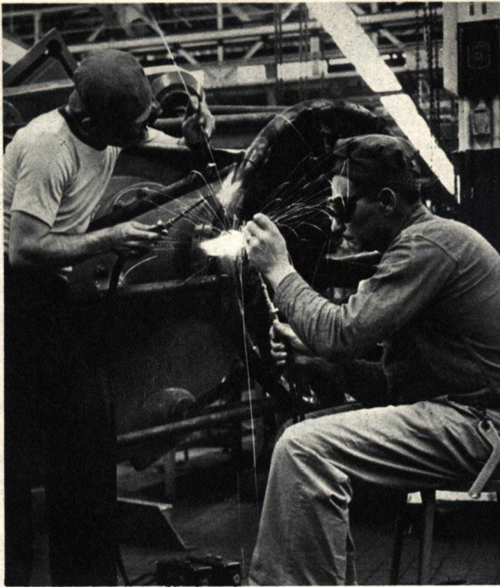
Skilled workers weld the motor mount with great care, for strength in this assembly is of great importance.
