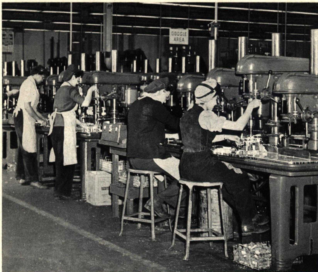
Linden drill press operators start a Wildcat on its way by drilling thousands of small parts which go into assemblies.
