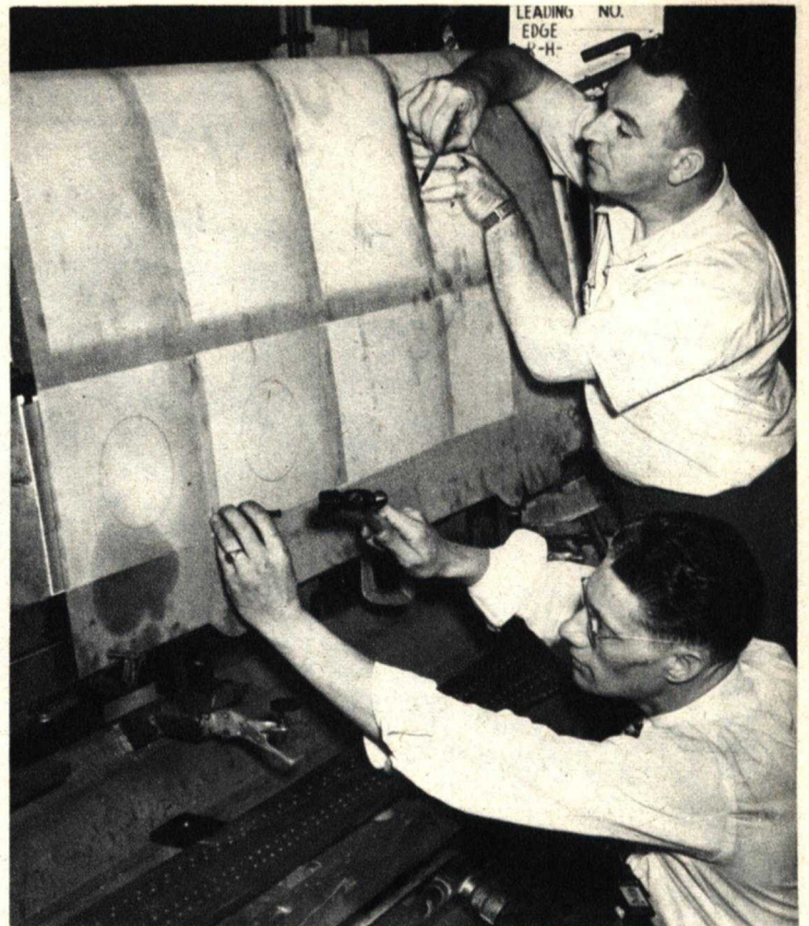
Holes in the skins of the leading edge are checked for accurate placement by a venilite master pattern.
