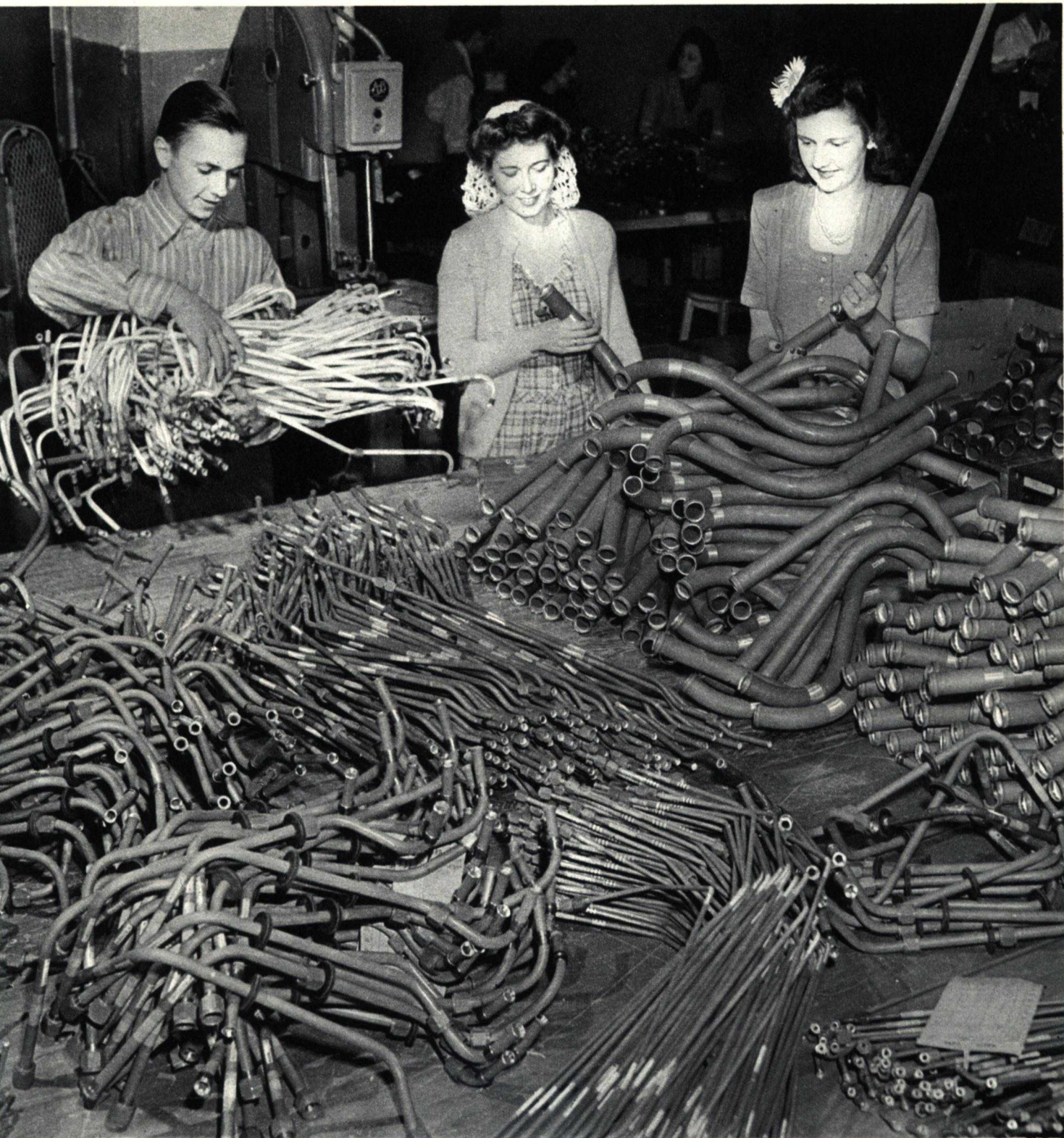
Air under pressure is shot through each tube to check for obstructions or imperfections. The ends are then taped, and the parts shipped to assembly plants. Many hundreds of these tubes go into each plane.
