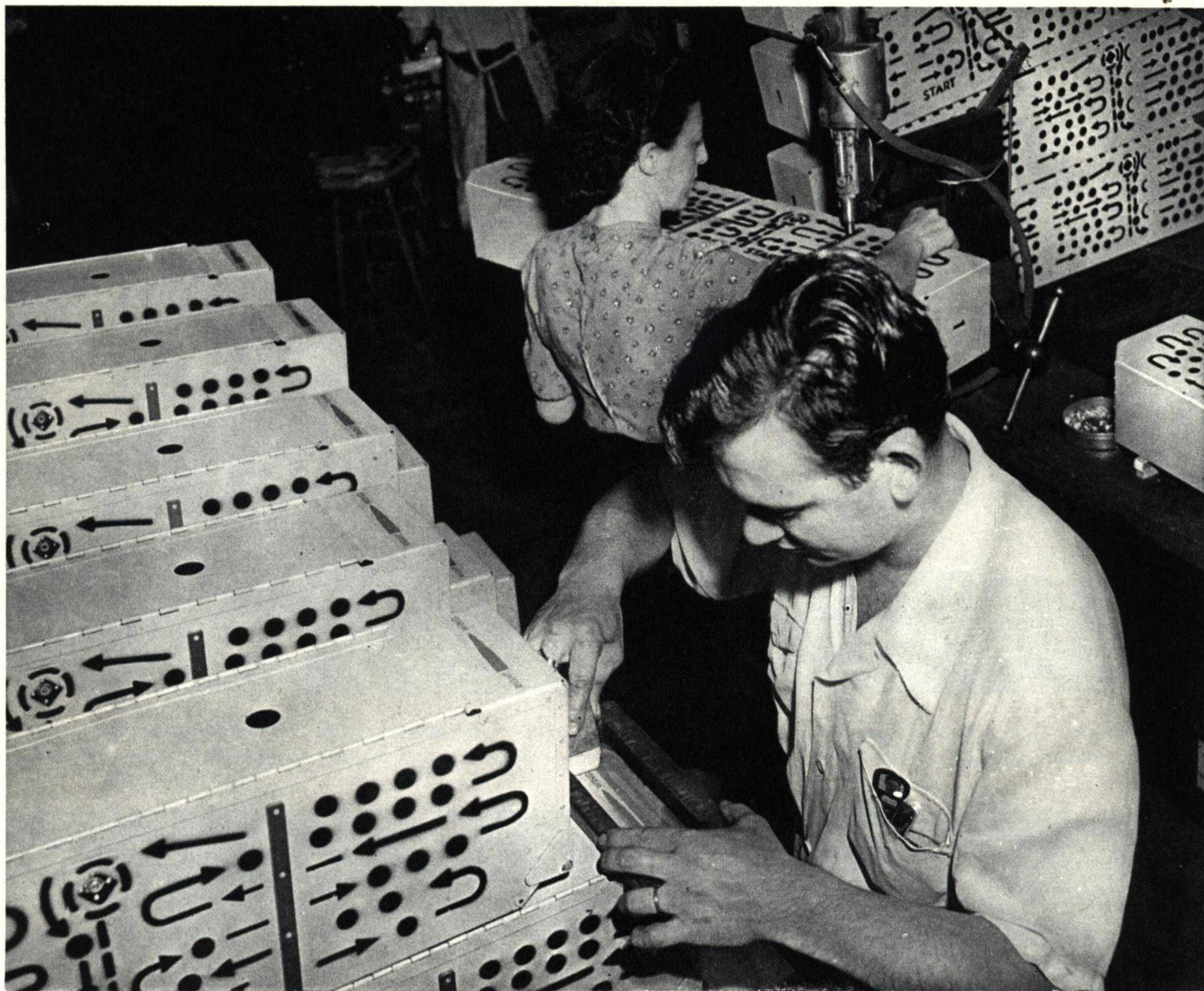
The boxes are finally stamped for proper installation in the plane. They are now ready to carry a load of ammunition into battle against the enemy. These boxes feed an even flow of bullets to the plane's guns.
