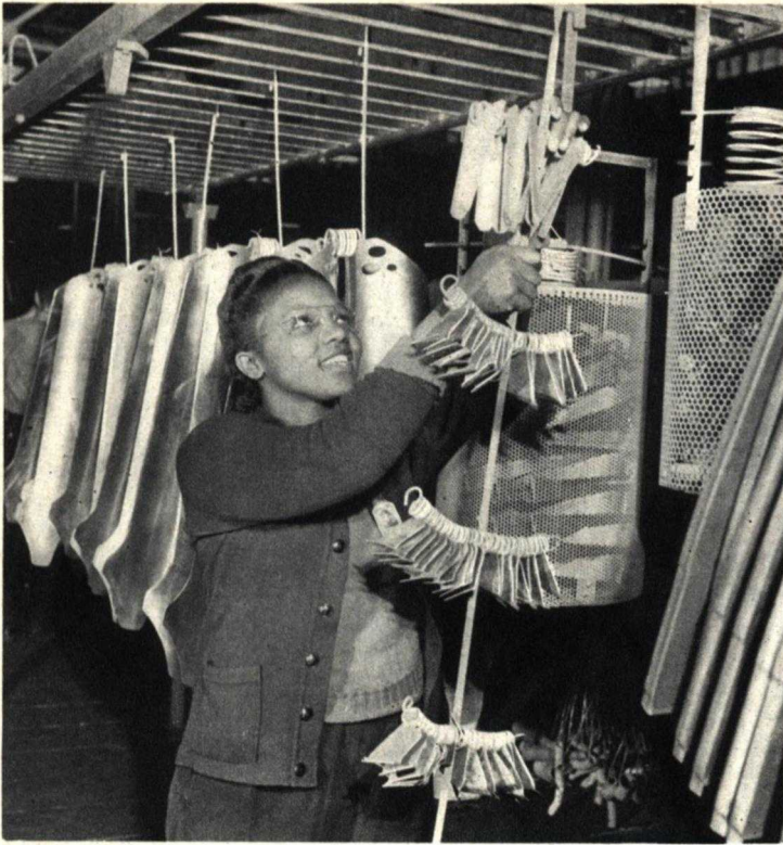
Racking them up! Parts, assemblies go on the dip rack for anodizing. This will retard salt-water corrosion.
