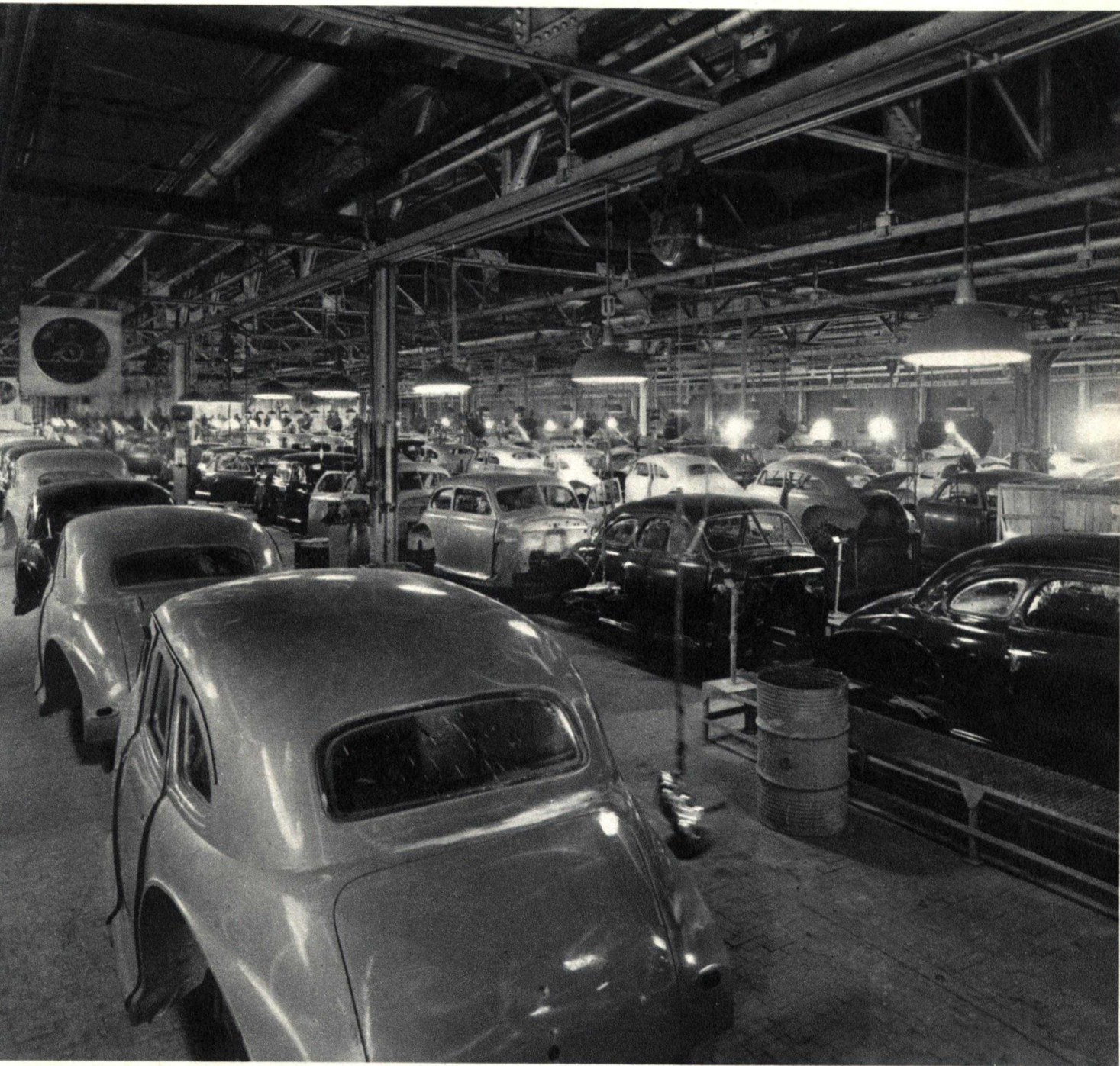
TRANSPORTATION WITHOUT WHEELS — Automobile bodies in various stages of completion passed in great quantities along the assembly lines of the Fisher Body Division plants in Baltimore and Tarrytown.
