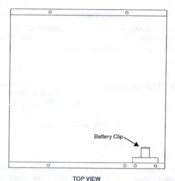
Snap the connector onto the battery and insert the battery into the mounting clip. Ensure that the connector leads are not free to contact any parts that move or conduct current.
