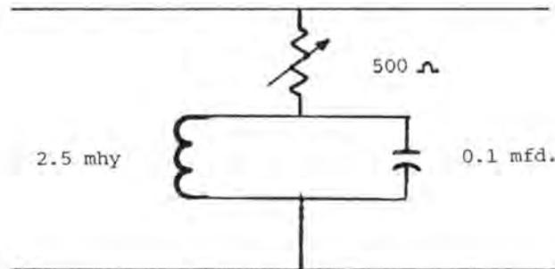
This equalizer is designed to maintain good response out to about 8kHz. This is accomplished by adding mid-band attenuation to bring down the mid-band response to equal that of the high end. This means that all passive equalizers, of necessity, increase overall line losses. Be sure the equipment on the other end of your audio line has the reserve gain to be able to work with the added loss.
