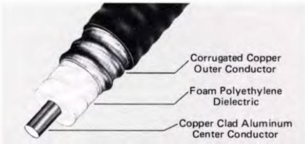
Cablewave Systems Foam Wellflex coaxial cables offer a combination of remarkable flexibility, high strength, and superior electrical performance. The designs include a copper clad aluminum center conductor, low-loss cellular polyethylene foam dielectric, corrugated copper outer conductor and a protective black polyethylene jacket. Foam Wellflex is used extensively in communications and electronic systems in the HF, VHF, UHF and microwave frequency bands.
