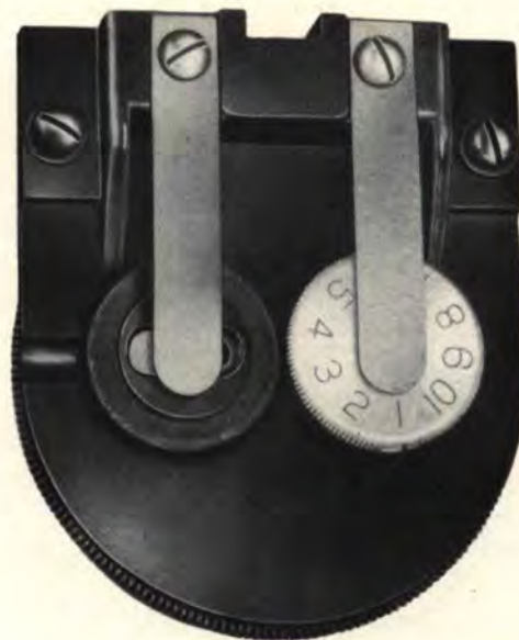
Fig. 3. Disks for Adjustment of Time Delay
