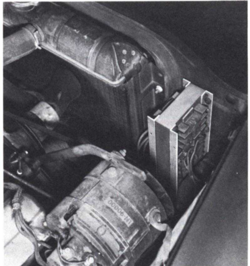
ENGINE COMPARTMENT VIEW of W8DLD's station wagon, showing Leece-Neville alternator in foreground and 3-phase distribution transformer mounted just ahead of it next to radiator.
