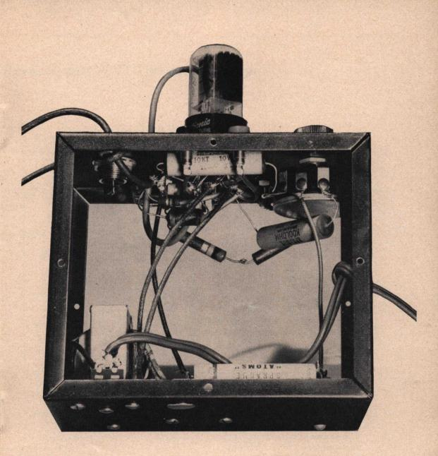
signal generator, an RF voltage of 4 volts read 3.8 volts with the Adapter-multi-meter combination. Above 10 megacycles the sensitivity fell off and the Adapter no longer gave an accurate reading. However, the presence of RF on the coil of a grid dip oscillator was still indicated by the Adapter up to 250 megacycles.
