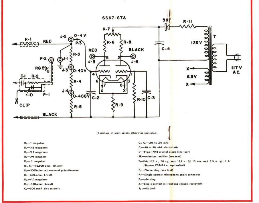
jack—this separate connector being provided to accommodate the coaxial cable and to permit the RF probe to be detached when not in use. If the DC test leads are wired into the circuit, as in the model illustrated, care should be taken not to allow the positive lead to touch a high-voltage spot when the RF probe is in use.
