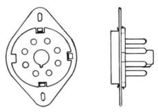
A few notes: Amphenol sometimes supplies a thicker mounting plate. Only the thinner ones can be used here. They seem to be the commonest kind. Also, a vise or pair of pliers can be used gently to push the base into the plate. It is a good snug fit.
