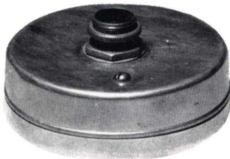
Fig. 6. Rear view of Electrophone showing microphone connector
