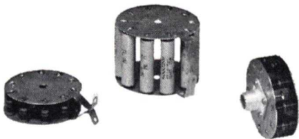
Fig. 13. Examples of parallel-connected resistors
