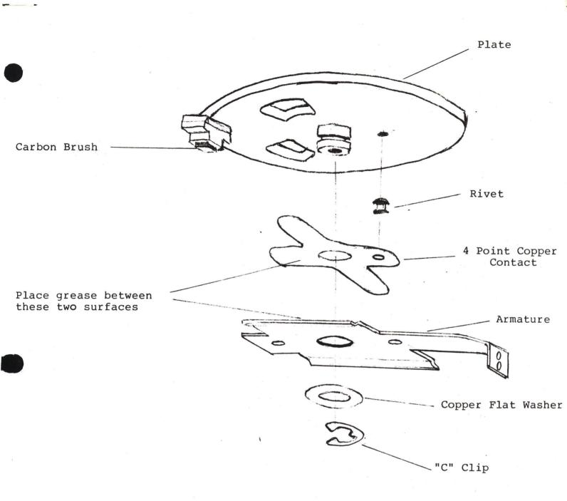
Plate Assembly for Variable Transformer, T2
