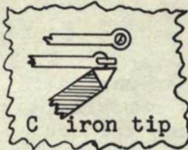
place the iron against the folded wire and rotate it away from the conductor leading into the fillet (2-c).
