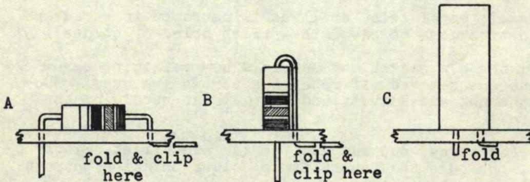
(A) & (B) Fold the leads on the new part to the same spacing as the mounting holes. Insert the part and fold the leads under the chassis to hold the part tightly against the top of the chassis. Clip off the excess wire.
