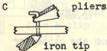
place iron on fillet again and pull the wire out of the hole on the top side of the chassis.
