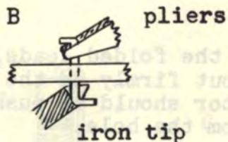
push wire through hole until hook can be clipped off.
