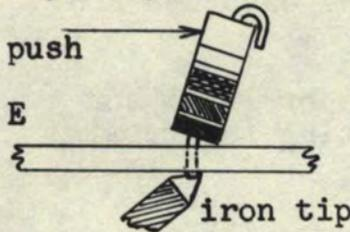
place iron on fillet again and push the resistor body over until the lead comes out of the hole.
