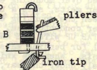
place iron on fillet and push wire through the hole until the hook can be clipped off.
