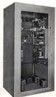
Rear view illustrates roomy design important in both servicing and low operating temperature. This is Gates walk-in design—average man can stand inside.
