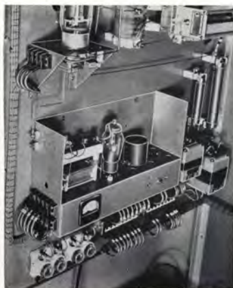
Oscillator unit holds two crystals and ovens and may be removed almost instantly for under chassis servicing.
