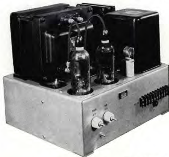
Above, left, the low voltage power supply deck. Right, the main high voltage supply delivering 2300 volts to power amplifiers and modulators.
