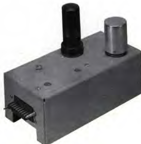
Below, left, illustrates three plug-in oscillator units in transmitter, ready to use. Right, individual oscillator removed for servicing, or exchange for another operating frequency.
