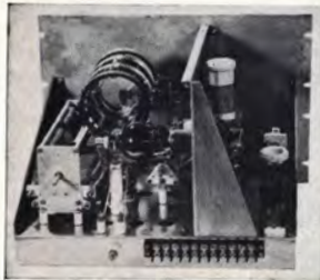
Above, radio frequency unit with plug-in coils. Below, modulator unit for use where above radio frequency unit is to be voice modulated.
