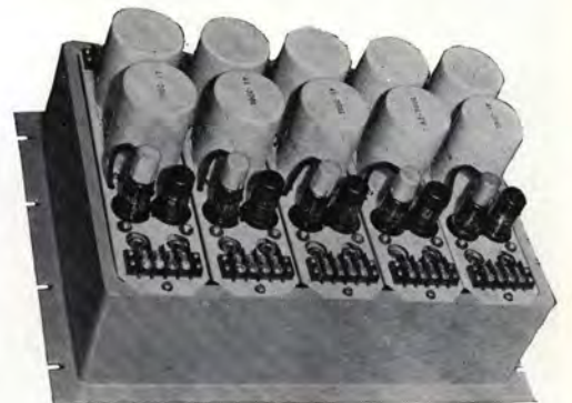
Figure E—Illustrates mounting five SA-70 preamplifiers on an SA-800 housing. This is the space saving and efficient way to mount Gates SA preamplifiers.
