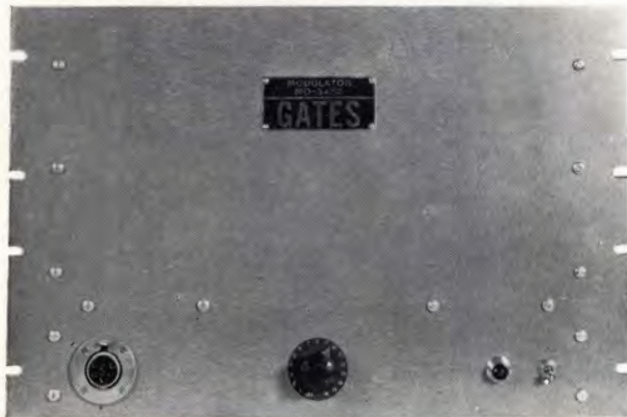
Above, radio frequency unit with plug-in coils. Below, modulator unit for use where above radio frequency unit is to be voice modulated.
