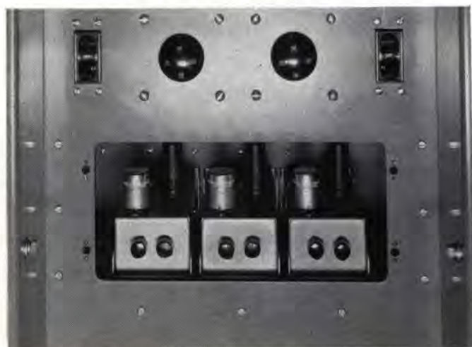
Below, left, illustrates three plug-in oscillator units in transmitter, ready to use. Right, individual oscillator removed for servicing, or exchange for another operating frequency.
