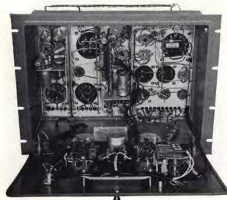
To service equipment mounted on SA housings, drop down the rigid cast front door. Note how every under-chassis component can be reached. Cabinet style strips need not be removed to drop down front door.
