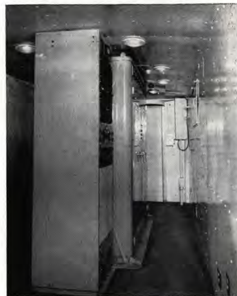
Indicating the rugged construction of the BC-1F transmitter is this mobile installation of the Armed Forces Korea network mounted in a six ton semi trailer van. Note the transmitter is firmly secured to floor with no snubbing connection to ceiling.
