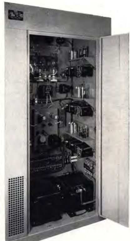
The right section of Gates HF1 series transmitter accommodates the entire audio system and intermediate power supplies. In telegraph models the audio system, of course, is not supplied.
