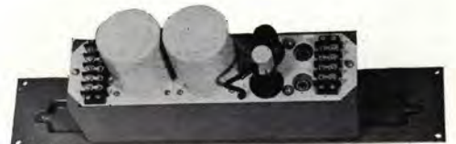
Figure D—Back view of SA-72 rack mount preamplifier. Note the shock mounting of tubes, test jacks for plate current, metering and isolation of input and output terminations.
