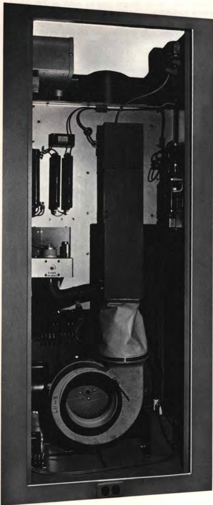
Rear view, visual power amplifier, BT-5H, 5 kW high band transmitter.
