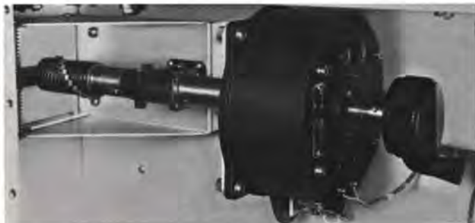
High torque DC servo motors direct coupled to PA circuits assure tuning accuracy. Reliability is enhanced through Gates design using fewer components.
