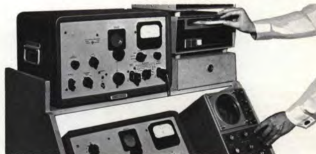
Each cartridge is tested for recovery level of recorded tone to assure stable levels from cartridge to cartridge.
