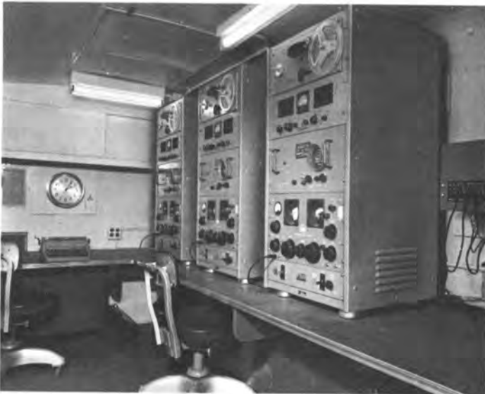
Mobile radio system designed and constructed by Gates for the Radio Bureau of the Republic of Korea provides complete medium and short wave broadcasting and public address facilities in a compact, specially designed van.
