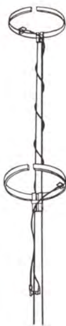
Left, FM-11 single ring omni-directional antenna with power gain of 0.8 dB. Right, two bay FM-22 omni-directional antenna with gain of 1.6 dB. These are broadband, easy to install antennas.
