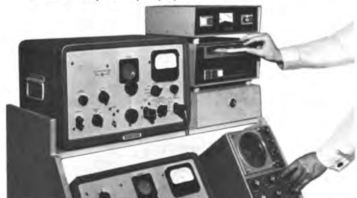
Each cartridge is tested for recovery level of recorded tone to assure stable levels from cartridge to cartridge.
