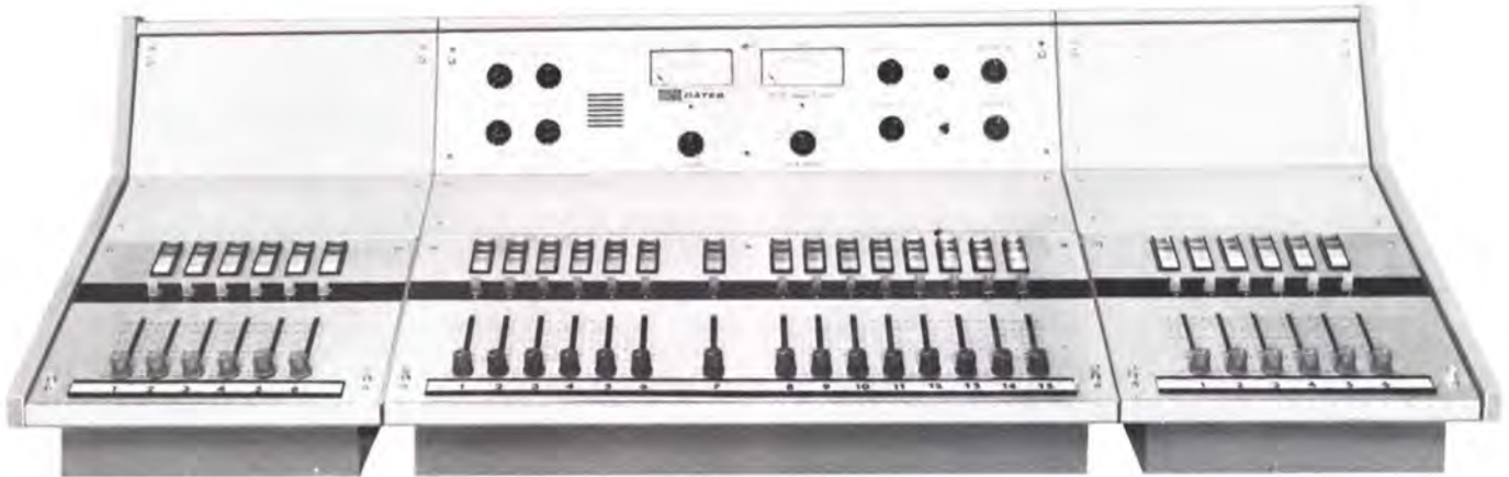
The TV-15 with two TVS-6 Sub-Mixer Units gives you 27 mixing channels and 108 inputs.
