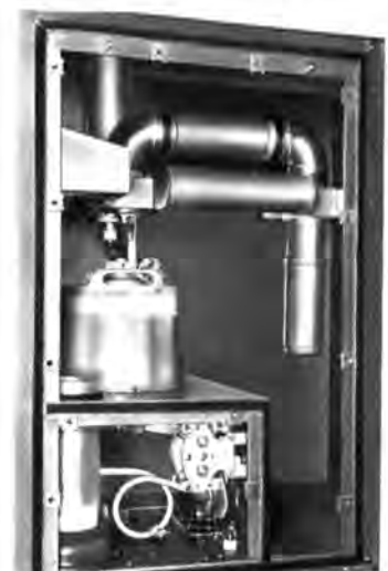
The Power Amplifier stage, which uses a 4CX15000A ceramic tube, has its driver amplifier located directly below for added efficiency of operation.
