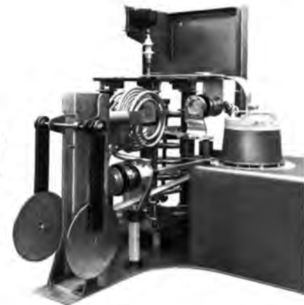
R.F. driver showing type 4CX15000 stage with grid circuits and cooling plenum.
