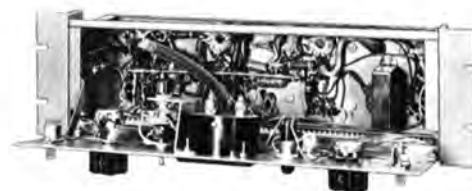
Right: Front panel drops down for easy servicing of all inner parts.
