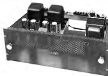
Dual plug-in program amplifiers and regulated power supply for TV-10 console. Standard rack mounting, 7" high, 14" deep.
