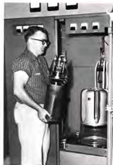
New F-8550 modulator tube weighs 65 pounds and only 90 pounds with socket assembly. Standardization on this new high power air cooled triode for both the modulator and power amplifier permits interchangeability of tubes for longer useful life. This reduces the number of tubes required as spares and lowers the cost of operation.
