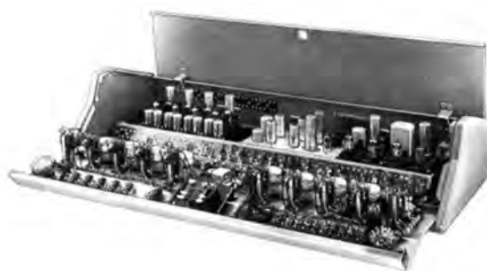
Open view showing complete accessibility.
