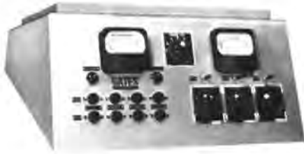
CCD-2 Transmitter control console.
