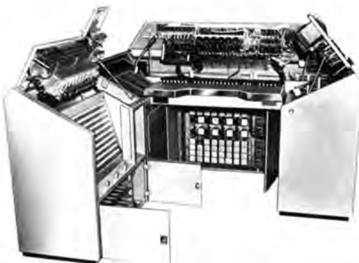
The above production console made for a leading television network houses 57 of the 6300 Series Solid Statesman transistorized units described herein.
