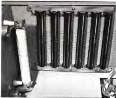
Inbuilt Dummy Antenna with 1 KW capacity handles full 100% modulation when used for testing the transmitter.
