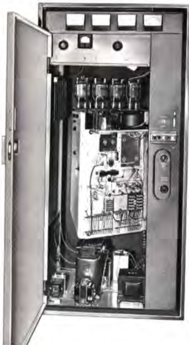
Completely self-contained, the BC-1G transmitter stands 78" high, 37" wide and 29" deep.
