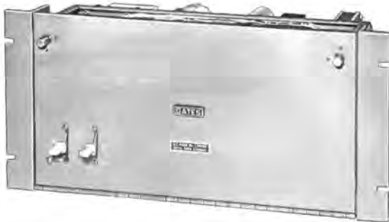
Fig. B Transmitter unit may mount in rack or small size permits mounting directly in most transmitters. Power supply is self-contained.
