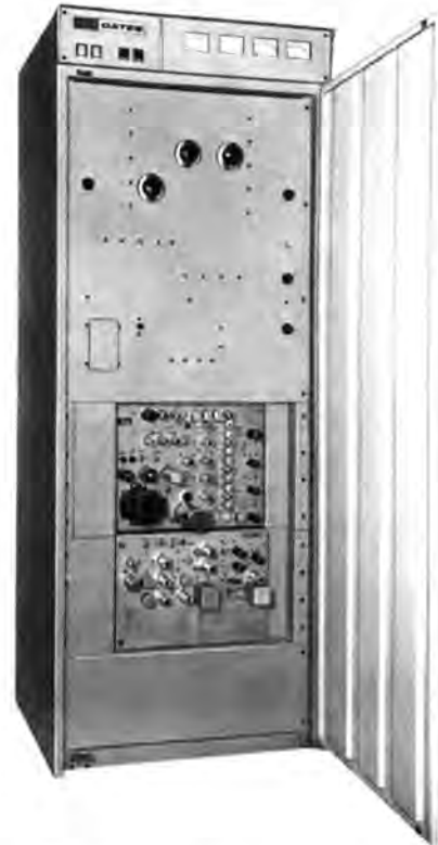
Front door open. The direct crystal controlled cascade exciter is illustrated above the stereo generating equipment below the cascade exciter. Note the two slip off panels below the stereo generator. Multiplex sub-channel generators fit here.
