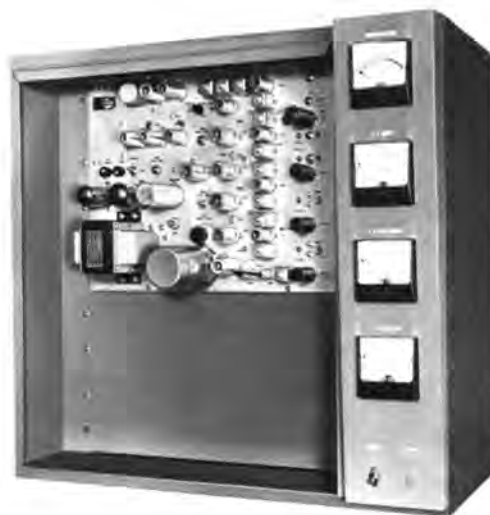
Front view (cover removed) of Model BFE-10C, ten watt FM transmitter. Models BFE-50C and BFR-50C are essentially identical in appearance.
