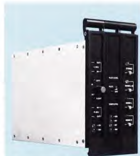
The Harris DSM Stereo Generator, with Digitally Synthesized Modulation (DSM) and DTR filter, provides 50 dB stereo separation minimum, 30-15,000 Hz, and overshoot no greater than 2%.
