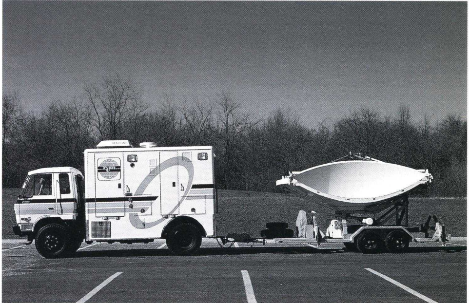
To meet length restrictions, the S-21Ts were built using a short-body design unit.
