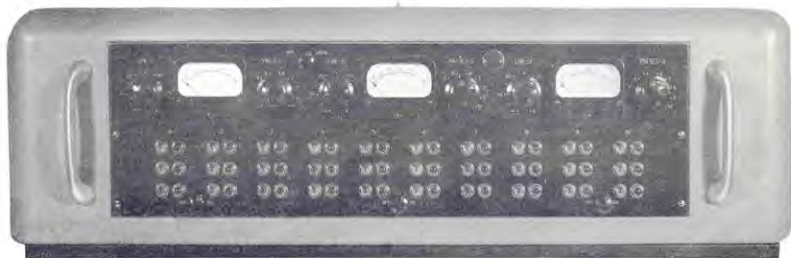
FIGURE A: The SA-110 master pre-set switching console exhibits extreme simplicity to control the most complex studio installation found in American broadcasting stations today.
