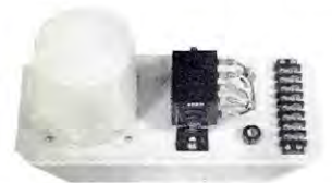
FIGURE B—The SA-108 DC power supply (rack panel not shown) which uses 5 \frac{1}{4} x 19 inches of rack space and delivers 6 volts DC at 4 amperes. Uses copper sulphate rectifier in full wave circuit.
