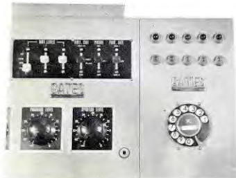
FIGURE C—A typical desk mounting is shown with the SA-106 dial circuit selector adjacent to a Gates 50-CS studio mic. The Gates dial circuit selector unit is in no way limited to use with Gates equipment only and is a completely self-contained, independently operating instrument.
