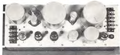
Illustrated above and below, the SA-98 two-watt monitoring amplifier with the exclusive Gates SA rack mounting feature for front-of-cabinet serviceability.
