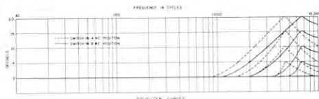
Typical curve of SA-118 equalizer for 4000 and 6000 cycles. Other frequencies are similarly covered.
