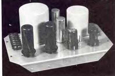
SA-95 ten watt monitoring amplifier illustrated above is another companion unit to the many space line amplifiers in the Gates audio line.
