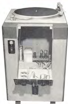
Figure B—The front section drops down for instantaneous accessibility of preamplifier and power supply tubes.
