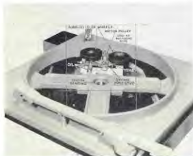
Figure A—Shear action of drive pulleys means drive pressure against air and is illustrated herein. To right, the speed change and master starting lever.
