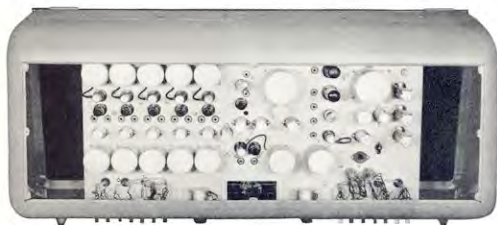
SA-40 Console looking from top. All preamplifier tubes are shock mounted. Note heavy sturdy construction of cabinet.
