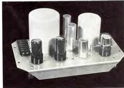
SA-96 two watt monitoring amplifier illustrates another compact yet highly convenient way of obtaining the most from rack cabinet space. SA housings described on Page 18 are suggested.
