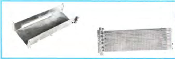
**F72531 (725 SCH) SINGLE CARD HOLDER**—Holds one 725 series card. Has card guides and mounting holes for F72541 or F72542 P-C Connector (not included). Mount up to (11) 725 SCH to 725 RM frame, or in custom INTEGRA 3 console shell. 3½" high x 11 7/16" wide x 7 5/8" deep.
