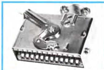
**F72543 (725 CFP) CONNECTOR, CHASSIS TYPE, MALE**—24 pin connector, with polarized barrier and keyed shell for mating with 725 CFS connector. Packaged complete with mounting hardware. (AMPHENOL, 26 series, BLUE RIBBON® connector)
