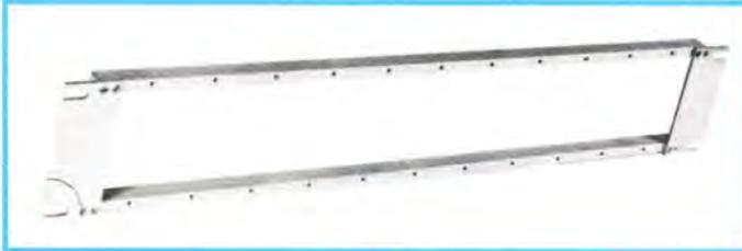
**F72530 (725 RM) RACK MOUNTING FRAME**—3½" high frame mounts in standard 19" rack. 16½" of mounting space with top and bottom rails drilled and tapped for #6-32 screws on 1½" centers. Holds up to (11) 725 SCH, or one 725 CFC.
