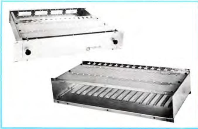
**F72514 (725 CFR) RACK MOUNTING CARD FILE**—Holds up to (16) 725 series cards, complete with card guides. Requires only 3½" of vertical space in standard 19" rack. Depth, 15". Features removeable front door and hinged rear panel with mounting provisions for (4) 725 CFP connectors and/or (8) UTC A series transformers and (4) 6-140-Y barrier strips. Mounting holes provided for (16) P-C Connectors (not included), No's. F72541 or F72542.
