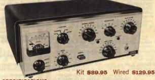
SPECIFICATIONS: Power Input: 90 watts CW (novice limit calibration on meter); 65 watts AM-phone with EXT plate modulation. Output Load Impedance: 50-1000 ohms. Band Coverage: 80, 40, 20, 15, 11, 10 meters. Operation: XTAL, EXT, VFO. Tubes: 1-6146 final amplifier, 1-6CL6 oscillator. 1-6AQ5 clamper, 1-6AQ5 buffermultiplier, 1-GZ34 rectifier. Power Requirements: 117 volts, 60 cycle AC. Size: (HWD): 5 "x 15" x 9". Shipping Weight: 30 lbs. Weight: 30 lbs.
