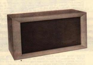
Extremely popular, high efficiency book-shelf speaker system kit supplied with fully assembled bass reflex cabinet ready for speaker mounting. All exposed surfaces smooth-sanded clear birch to permit easy and attractive finishing. 8" woofer has powerful ½ lb. slug magnet. Compression driver tweeter loaded by cast aluminum horn. Response engineered for smooth crossover at about 2000 cps. Bridging capacitor crossover with tweeter level control.
