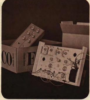
Chassis has all jacks, sockets terminal boards, transformers pre-mounted.
