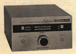
Incorporating the best features of matrixing and sampling techniques, the MX99 automatically delivers stereo or mono from the appropriate signal without being touched. An indicator lamp turns on when the station selected is broadcasting multiplex stereo.
