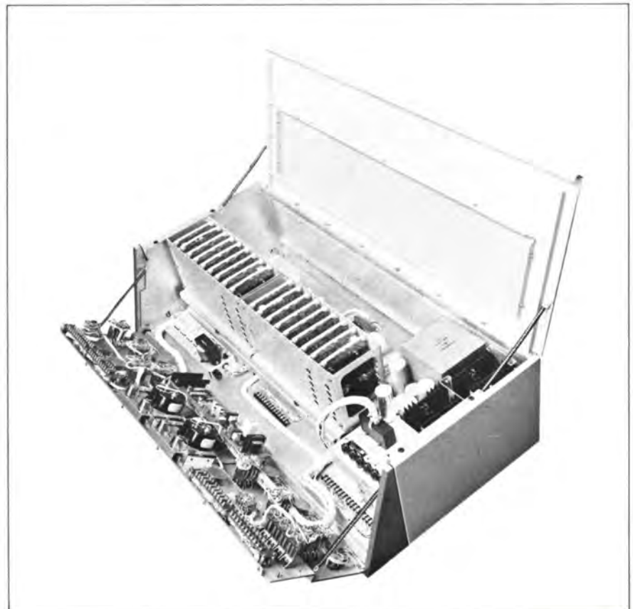
External and opened configuration of 212S-1, showing easy accessibility of its components.
