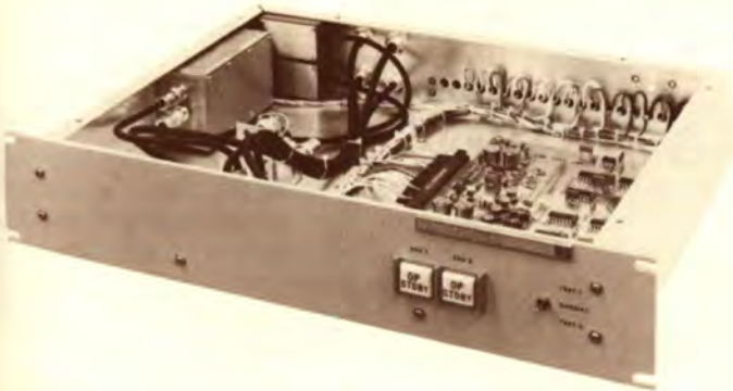
377C-1 Automatic Exciter Switcher
