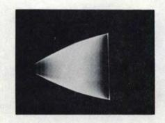
Figure 3-5. Incorrect Phasing, as Indicated by a Trapezoidal Pattern
