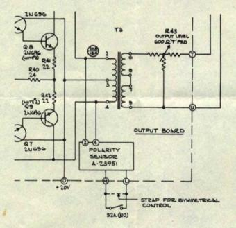
To install this new Polarity Sensor, remove the present one on the Output Board, and replace it with this new version. When soldering, make sure the points M, L, 2 and 4 are properly positioned. See drawing above; also refer to page 4-4 of your Volumax manual.
