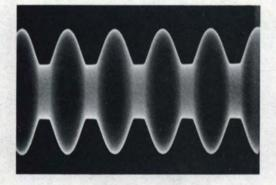
Figure 3-1. Correct Phasing, as Indicated by Intentionally Overdriven Volumax
