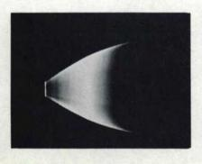
Figure 3-4. Correct Phasing, as Indicated by a Trapezoidal Pattern
