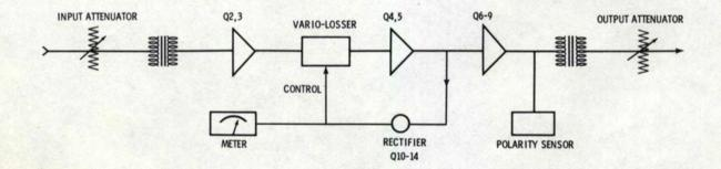
Figure 4-1. Volumax - Block Diagram
