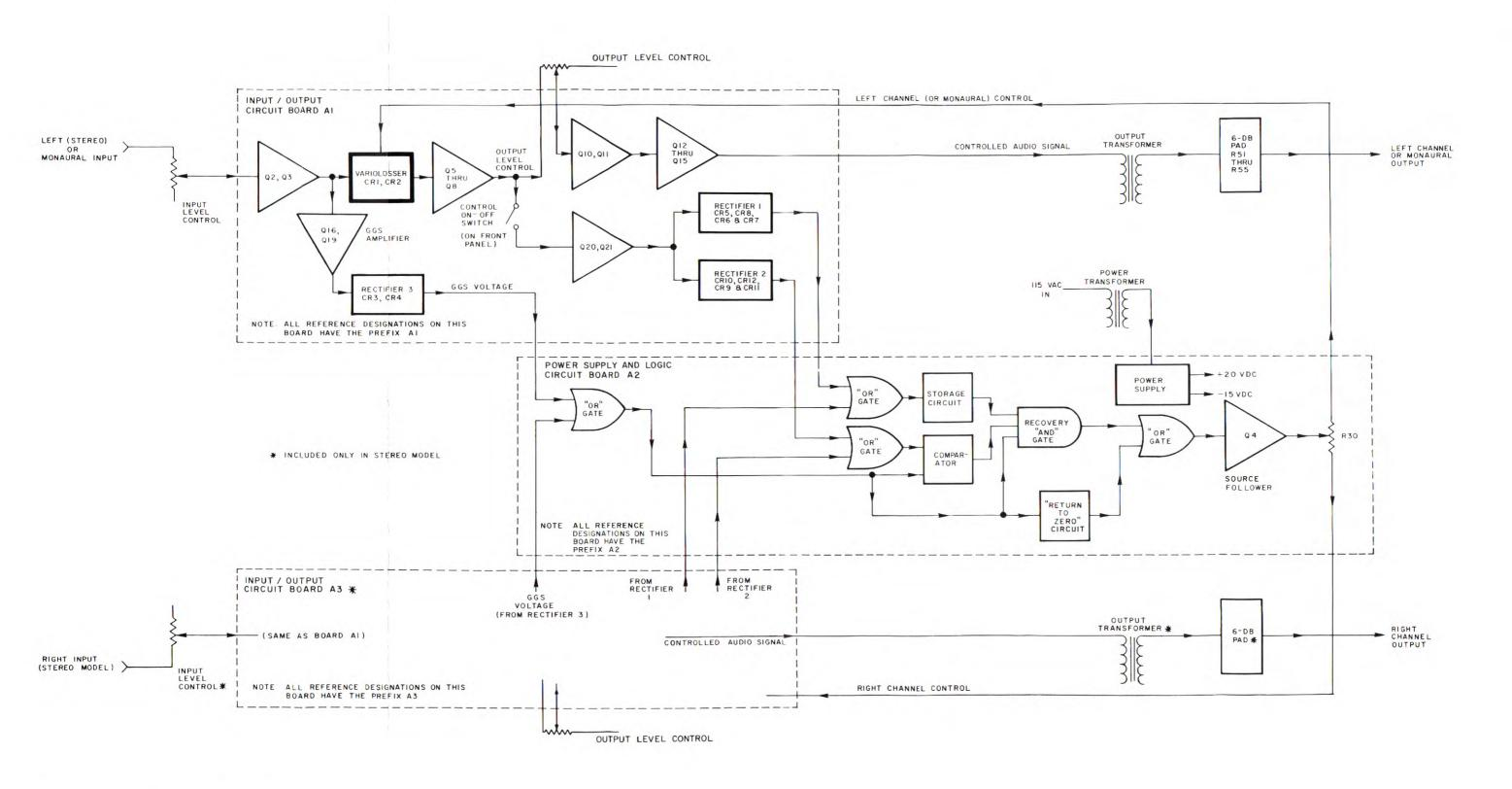
Figure 4-1. Audimax Block Diagram
