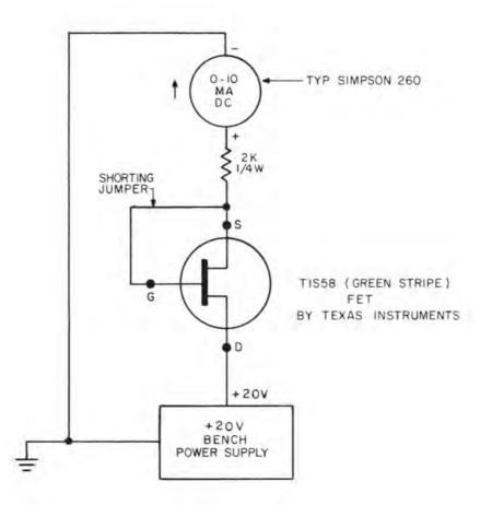
Figure 5-2. I<sub>dss</sub> Bench Test Circuit for T1S58 (Grn Stripe) Replacement of A2Q4
