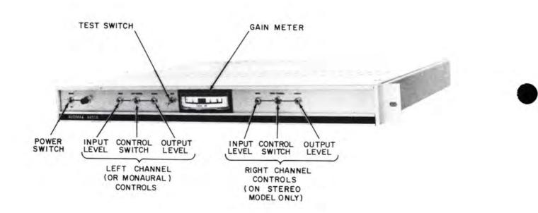
Figure 3-1. Audimax Unit, Front Panel Controls
