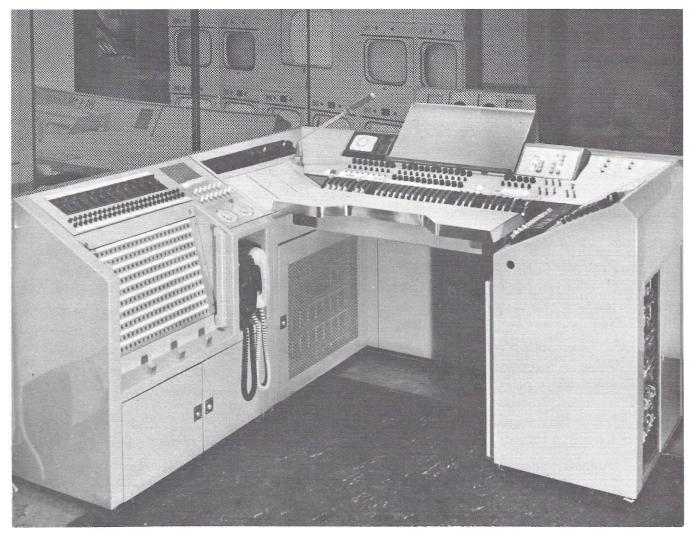
FIGURE 5-5. A self-contained studio audio console of the wrap-around type.
