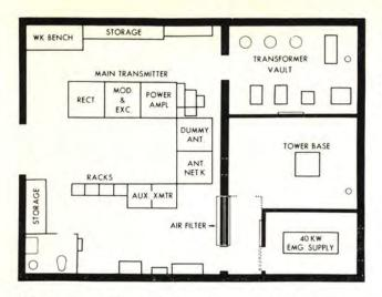
Fig. 3 KNX floor plan.
