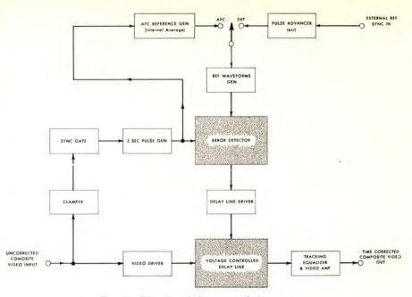
Fig. 5—Functional diagram of the Amtec.
