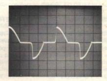
9. Stereo Demodulator Waveform, No Modulation
