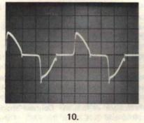
Stereo Demodulator Waveform, Incorrect Balance
