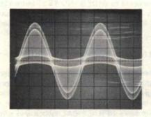
4. Composite Stereo Waveform, Insufficient (L-R)
