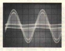
6. Composite Stereo Waveform, Phase Error Between (L+R) and (L-R)
