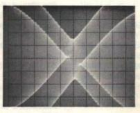
8. (L-R Subcarrier with Pilot, Pilot Phase Incorrect
