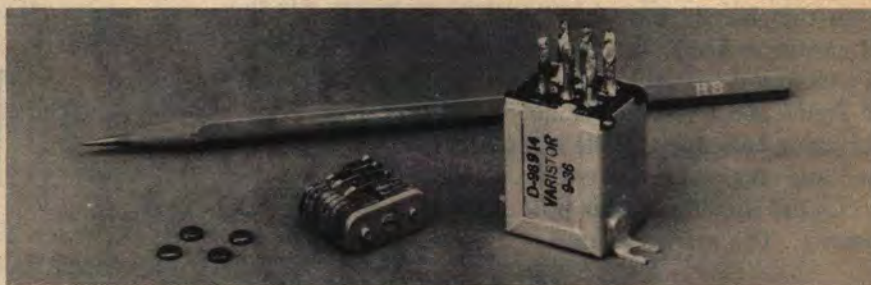
COPPER-OXIDE VARISTOR UNIT USED AS MODULATOR AND DEMODULATOR
