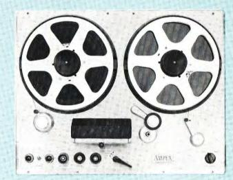
Tape transport Three precision, heavy duty motors handle reels up to 14 inches in diameter, tapes up to 1 inch in width (the Ampex Series 300 are the only recorders that will accommodate more than one-half inch tape). Flutter and wow have been virtually eliminated due to rigid unit assembly, carefully designed precision capstan drive, massive flywheel and longer tape path. Tape skewing is non-existent; starts and stops are instantaneous.
