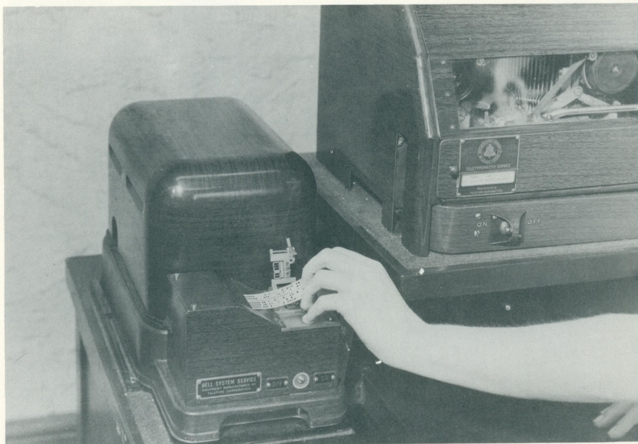
This is tape sending. The operator is shown feeding the perforated tape into the automatic transmitter.
