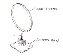
(5) Orient the AM loop antenna so that the best reception is obtained.
