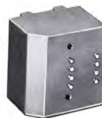
Dual saturable reactor. Input 10 V. - 1 kHz. Output 3.5 V. 2 MA DC control current. 130° C. MIL-T-27C; 1¾ x 1¾ x 1¼, 5 oz.
