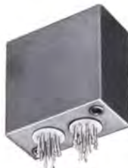
Precision reference transformer. Input 14 V., 400 Hz. Twelve secondaries held to low phase shift and .1% tolerance MIL-T-27C; 1¾ x 2 x 1¾, 4.5 oz.
