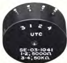
Toroidal transformer, primary 600 ohms, secondary 1200 ohms/split. From 1 kHz to 150 kHz, ±1 db at 10 mw max. Size: 1 1/8 Dia. x 3/8 inches. Weight: 25.6 grams. All types of toroidal transformers to specific requirements.
