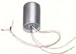
Microphone input transformer, double drawn Hipermalloy shields. Shielded cable leads. Ratio 100:1. 1 3/16 Dia. x 1 1/32" high. Inductance greater than 1000 Hys. at 60 Hz.
