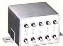
Thirty Hz cathode follower output transformer to provide equal voltages to 4 loads and supply a half-wave rectifier. Primary inductance maintained to 5% with 20% change in DC unbalance and 30% change in AC voltages.
