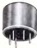
Molded carrier frequency transformer, + 8 dbm level. Within 3 db from 100 Hz to 100 kHz. 4000:4000 ohms. 3/4 Dia. x 5/8 inches, 1/3 oz.
