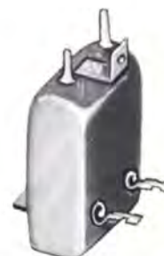
RF saturable inductor. 2 MA DC for sweep from 17 MHz to 21 MHz. MIL-T-27C; 2 oz.
