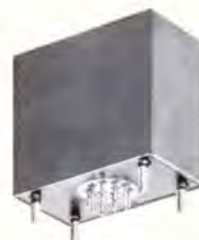
Bolometer transformer. Primary 10 ohms, secondary 530K ohms, 230:1 ratio, response from 1/2 Hz to 25 Hz. 120 db magnetic shielding, to 25 Hz. 120 db magnetic shield-plus full electrostatic shielding.
