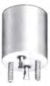
High Q, 5 millihenries inductor. High Q in the 10 kHz to 300 kHz frequency range. Grade 4, MIL-T-27C. Weight approximately 1.5 oz.
