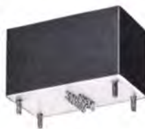
Precision Magnetic Modulator and Filter to produce sine wave output directly proportional to a DC control input. Temperature stabilized from -55°C to 85°C. Distortion and linearity less than 3% thru temperature and frequency range of 380-420 Hz. MIL-T-27C, 1½ x 1½ x 3½", 12 oz.
