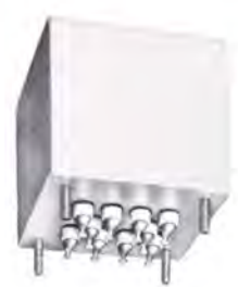
High voltage, constant inductance, tapped inductor. 16 millihenries, 8 kHz, inductance variation less than 1% from 1 volt to 1600 volts. Q greater than 40 at 1600 volts. Case size: 3 1/8 x 3 1/8 x 2 3/4" high. Grade 4, MIL-T-27C.
