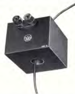
Current Transformer with 1 K load exhibits 1 V/amp/turn sensitivity. From 400 Hz to 30 kHz, ±0.1 db. Good linearity with both current, 1 mA-10 A; and turns, 1-5 T.
