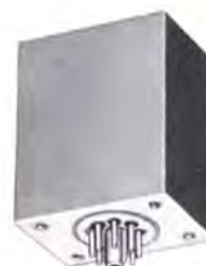
Magamp for 11 watt, 115 V., 400 Hz servomotor. Standard octal plug. MIL-T-27C; 1¾ x 2½ x 3, 1.7 lb.
