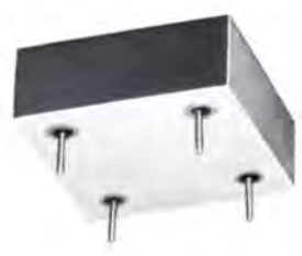
Flat low frequency 50 henries inductor only .400 high. Q of 10 at 100 Hz. DCR 2360 ohms. Grade 4, MIL-T-27C.
