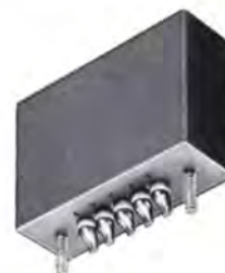
Saturable reactor. Input 50 V.-60 Hz. Output 10 V., 4 MA DC control current. MIL-T-27C; 7⁄8 x 2½ x 1½, 6 oz.
