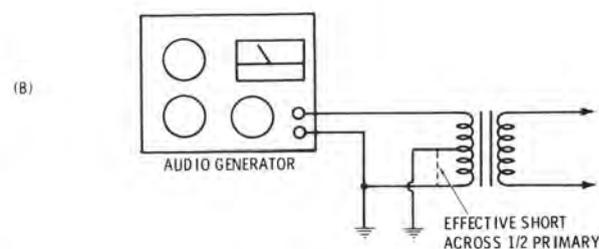
Direct connection across a truly balanced input can result in severe mismatching and test conditions not simulating normal operation of the input circuit.
