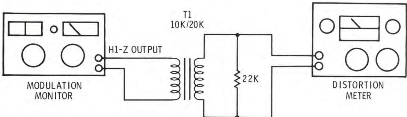
**Figure 5.** A simple high impedance isolation circuit. Note that the secondary winding of the transformer is loaded with a resistor equal to the secondary impedance. The modulation monitor output impedance will usually be low enough to load the primary, but the 100,000
