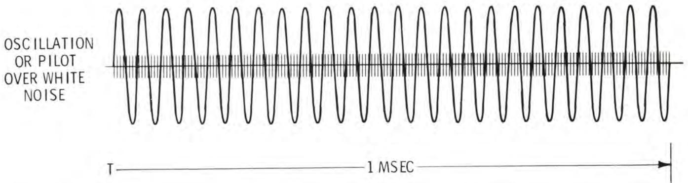
If the noise is a high frequency oscillation, the scope sweep can be adjusted to lock in on the signal. White noise is random in nature and can not be "synced".
