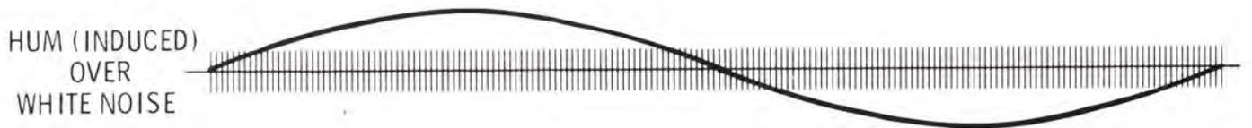
Hum pickup is easy to identify because the pattern will lock when the scope sweep is synchronized to the line voltage.
