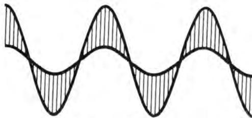
Wavy baseline in this direction shows excess L+R or too little L-R. Adjust either level for straightest baseline.
